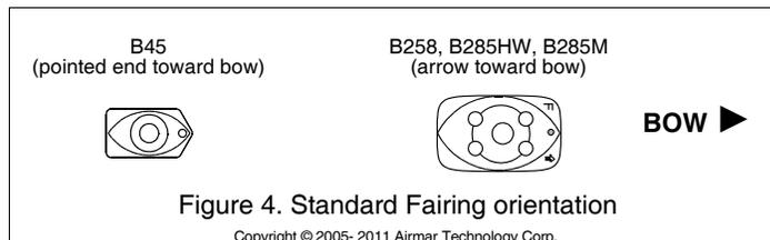
*facing forward toward the bow. The long side must be parallel to the centerline of the boat (Figure 4).*
